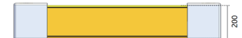
Ground barriers Impact protection for forklifts. Both horizontal and arcuate ground barriers are available.
