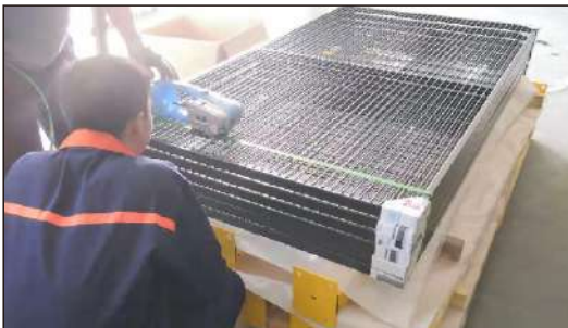
Corner protection to protect each panel from abrasion, five pieces in one bundle
